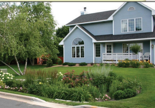
Rain gardens are shallow depressions that capture and treat stormwater naturally. Photo credit U.S. Environmental Protection Agency
